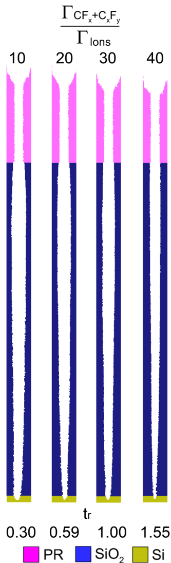
FIG. 13. Final etch profiles (central slice) with 10% over-etch of during HAR etching for different (CF_x + C_xF_y)/ion flux ratios from 5 to 40. Only PR, SiO 2 , and Si are shown, with the complex and polymers being blanked out. The (CF_x + C_xF_y)/ion flux ratio in the base case is 30. The fluxes of ions were varied, while the fluxes of CF x and C x F y remained constant. The same IEADs from the base case were used in all cases. The relative etch time, t_r , is listed below each feature.
