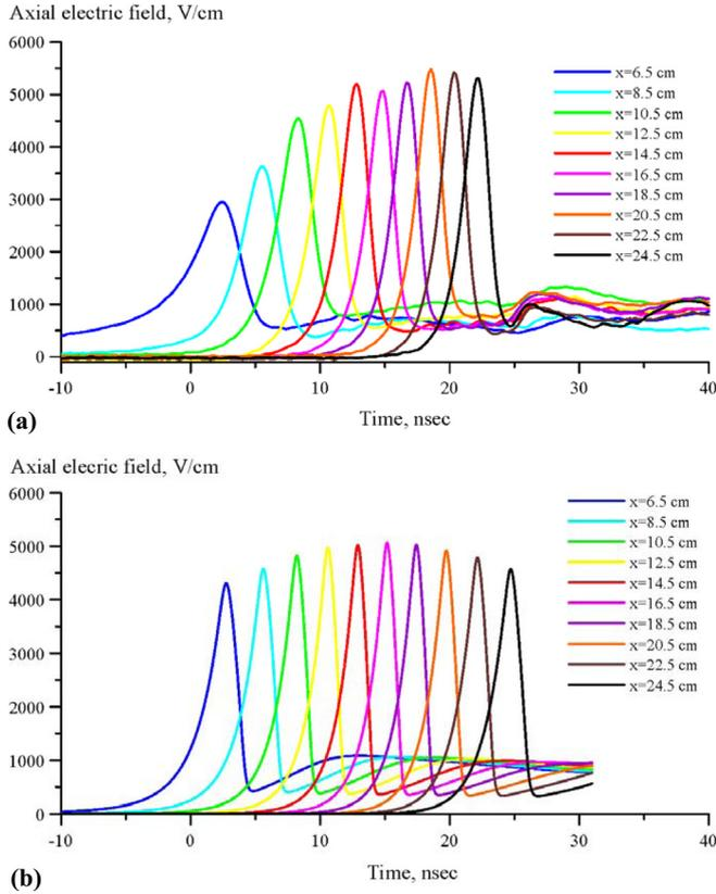
FIG. 12. (Color online) Comparison of (a) experimental and (b) predicted time-resolved axial electric field at different distances from the high-voltage electrode at the conditions of Fig. 10(a) (positive polarity wave). Numerical calculations using a quasi-one-dimensional FIW discharge model.
