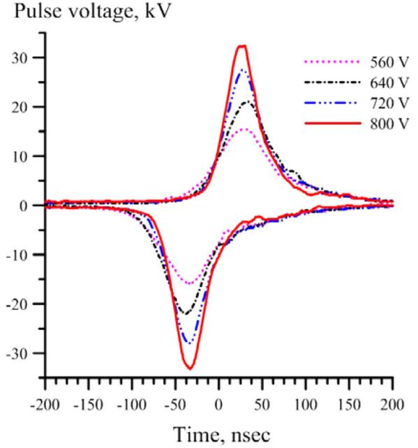
FIG. 2. (Color online) Typical positive and negative polarity voltage pulse waveforms generated by the pulsed plasma generator for different input DC voltages.
