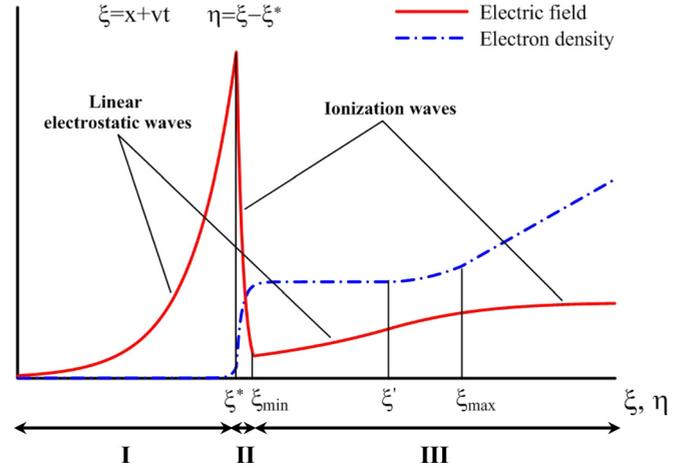
FIG. 16. (Color online) Schematic of a quasi-one-dimensional ionization wave structure.
