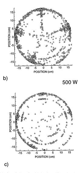
FIG. 7. Plan (or top) views of particle locations while varying plasma operating conditions: (a) 100 mTorr, (b) 200 W power deposition, and (c) 400 W power deposition. Traps are more closely aligned with the nozzles at higher pressure. The traps are dispersed at the higher powers, first at the mid-nozzle locations and load-lock bay, and later at the nozzle locations.
