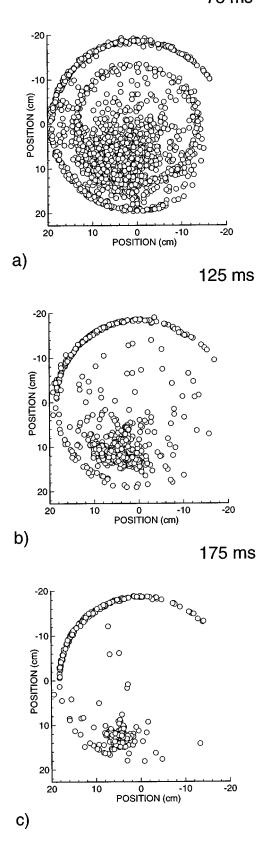
FIG. 11. Plan (or top) views of particle locations (1  $\mu$ m diameter) in the solenoid ICP reactor at various times after release: (a) 75 ms, (b) 125 ms, and (c) 175 ms. Particle trapping occurs at the azimuth corresponding to the minimum in power deposition.
