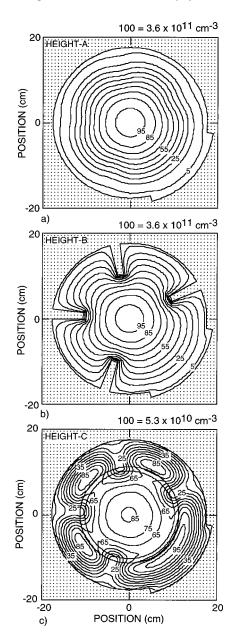
FIG. 3. Ion density for an Ar discharge at 10 mTorr in the  $(r, \theta)$  plane at the heights indicated in Fig. 1: (a) below the window (height A of Fig. 1), (b) at the nozzles (height B), and (c) above the wafer (height C). Contours are labeled with the percentage of the maximum value shown in each figure. The ion density is significantly perturbed near the wafer due to both recombination on the nozzles and a shadowing of ion sources at higher heights.
