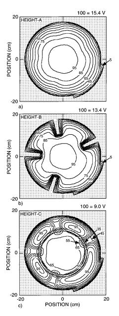
FIG. 2. Plasma potential for an Ar discharge at 10 mTorr in the  $(r, \theta)$  plane at the heights indicated in Fig. 1: (a) Below the window (height A of Fig. 1), (b) at the nozzles (height B), and (c) above the wafer (height C). Contours are labeled with the percentage of the maximum value shown in each figure. The plasma potential is perturbed many cm from the nozzles.
