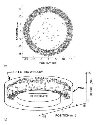
FIG. 4. Particle locations (1  $\mu$ m diameter) in an ICP reactor without nozzles: (a) plan view from the top and (b) cut-away view. Particle traps occur only in the peripheries and corners of the reactor where ion fluxes have decayed to low values.
