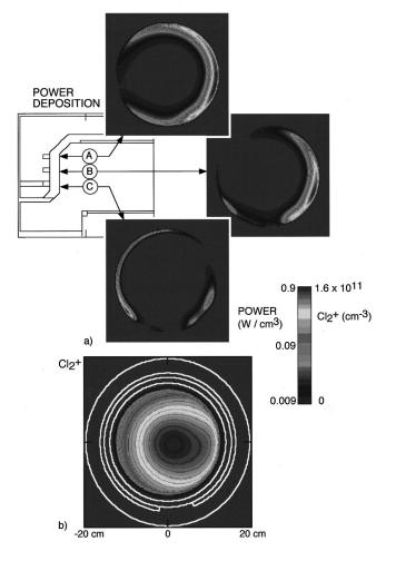
FIG. 10. Plasma properties of the solenoid ICP reactor (10 mTorr Cl<sub>2</sub>, 400 W). (a) Power deposition in the  $(r, \theta)$  plane for heights approximately aligned with the coils. Poor impedance matching produces azimuthal variations. (b) Cl<sub>2</sub><sup>+</sup> density in the  $(r, \theta)$  plane at height C. The ion density has an azimuthal maximum aligned with the power deposition.
