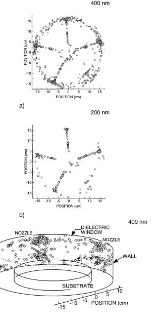
FIG. 8. Plan (or top) views of particle locations for: (a) 400 nm and (b) 200 nm diam particles. A cutaway view in (c) shows locations of 400 nm particles. Trapping occurs above and below the nozzles, and at the tip.
