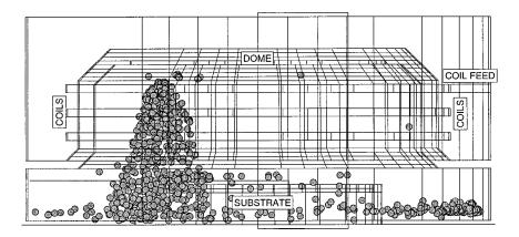
FIG. 12. Side view of particle locations at 175 ms for the conditions of Fig. 11. The particle trap extends from the bottom of the reactor into the dome, narrowing at larger heights.
