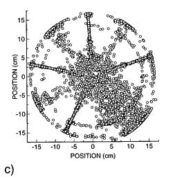
FIG. 5. Plan (or top) views of particle locations (1  $\mu$ m diameter) in the ICP reactor with nozzles and a load lock bay at various times after release: (a) 25 ms, (b) 100 ms, and (c) 175 ms. Particle trapping occurs in the bulk plasma at azimuths aligned with the nozzles, at midpoints between the nozzles and in front of the load-lock bay.
