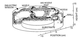
FIG. 6. Cut-away view of particle traps 175 ms after release for the conditions of Fig. 5(c). Particle traps are produced above and below the nozzles, as well as in front of the tip of the nozzle.
