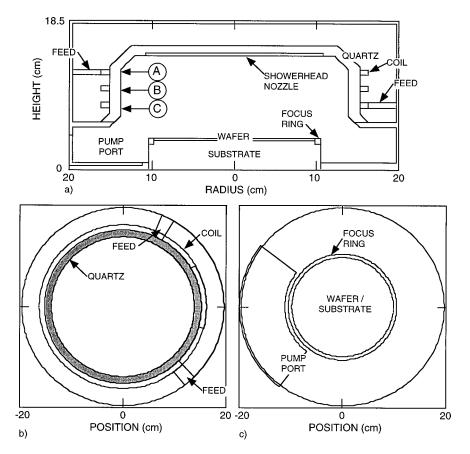
FIG. 9. Schematic of the solenoid coil ICP reactor: (a) side view, (b)  $(r, \theta)$  slice through the dome showing the coil and feed locations, (c) view looking down on the substrate. The arrows in the top figure indicate the heights at which  $(r, \theta)$  "slices" of plasma properties will be viewed.
