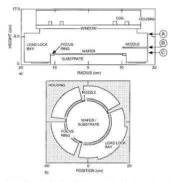
FIG. 1. Schematic of the flat-coil ICP reactor having injection nozzles used in this study: (a) side view, (b) view looking down on the substrate from below the window. The four nozzles extend to the edge of the wafer. The arrows in the top figure indicate the heights at which  $(r, \theta)$  "slices" of plasma properties will be viewed.
