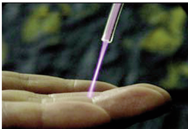
An atmospheric plasma flows onto a hand without causing injury.
