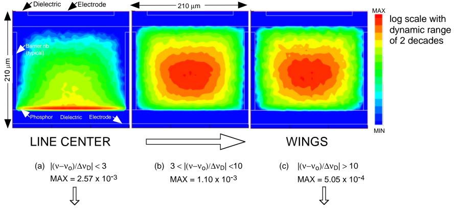
Photons with v ~ v<sub>o</sub> are more likely to be emitted near the phosphor  Photons emitted from the wings are more likely to originate in the center of the PDP cell where the Xe\* density is greatest
