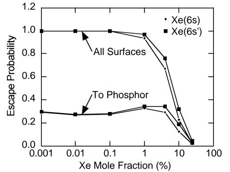
• Escape probabilities as a function of Xe concentration for primary UV photons emitted by the resonant transitions:
