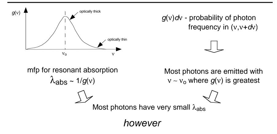
There is a small probability that the photon will be emitted from the wings of the line shape where the cross-section for resonant re-absorption is low
