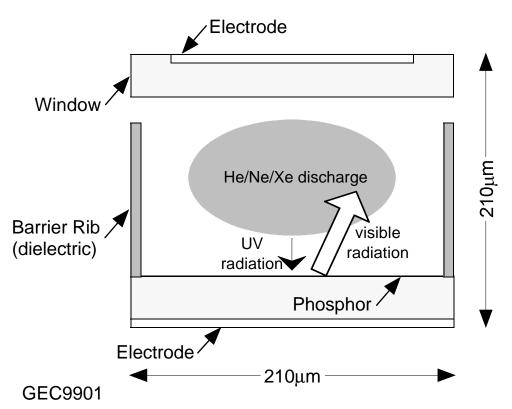
• Schematic of PDP cell.
